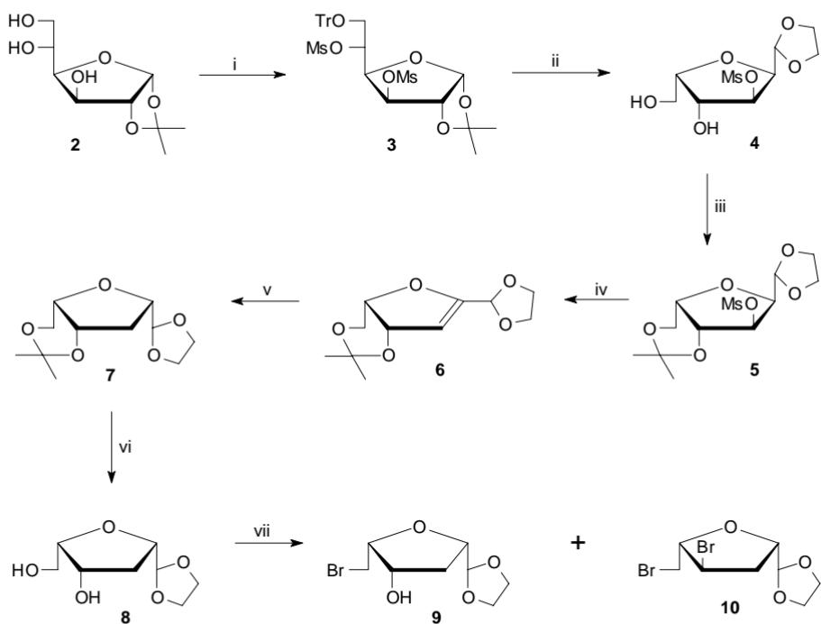
(i)  $\text{TrCl}$ , Py, rt, then  $\text{MsCl}$ ,  $+4^\circ\text{C}$  (100%); (ii) Ethylene glycol,  $\text{TsOH}$ , benzene, reflux (51%); (iii)  $\text{Me}_2\text{C}(\text{OMe})_2$ ,  $\text{TsOH}$ , rt (87%); (iv)  $\text{Bu}_4\text{NF}$ , MeCN, reflux (76%); (v)  $\text{H}_2/\text{PtO}_2$ , EtOH, rt (94%); (vi)  $\text{CF}_3\text{COOH}$ , MeOH, rt (79%); (vii)  $\text{CBr}_4$ ,  $\text{Ph}_3\text{P}$ , Py, rt (23% of **9** + 24% of **10**)
